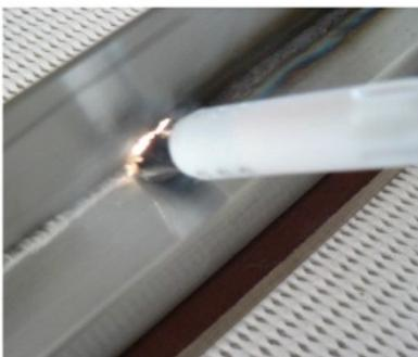
**TEKTIG** introduces the **KSS** Weld Cleaner **Sliding Shroud**. The **KSS** is a revolutionary and practical new invention, it is easy to use, making weld-cleaning safer and quicker, a definite must for all professionals. The **KSS** performs three main functions; it confines the bristles to ensure that you clean what you want and not where the bristles point to; it acts as a reservoir for the electrolyte and **Reduced Spills**; and it extends the lifetime of the brush by as much as 200%.
